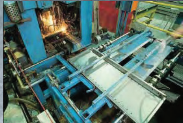
Automatic shelf welding on Hi-Performance shelf production line.
